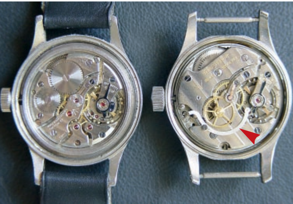
The IWC (cal 89) and Jaeger LeCoultre (cal 488/sbr) watches produced to the MoD's Mk 11 specification. On the JLC the hacking feature can be seen, arrow.
