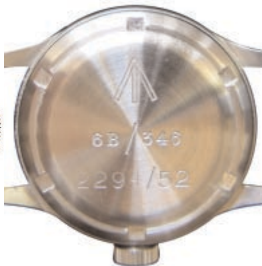
Examples of the military markings on Mk 11 watches. The arrow denotes Government Property, 6B/346 refers to a watch meeting the Mk specifications. The lower number is a serial number followed by the two digit year in which the order was placed with the manufacturer.
