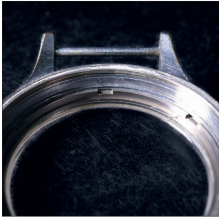
Figure 5A. Screw down ring to tighten the crystal, Record w.w.w.
