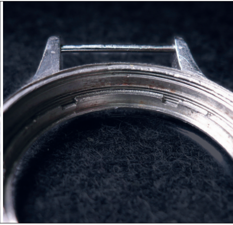
Figure 5B. Screw down ring to tighten the crystal, IWC Mk. 11.
