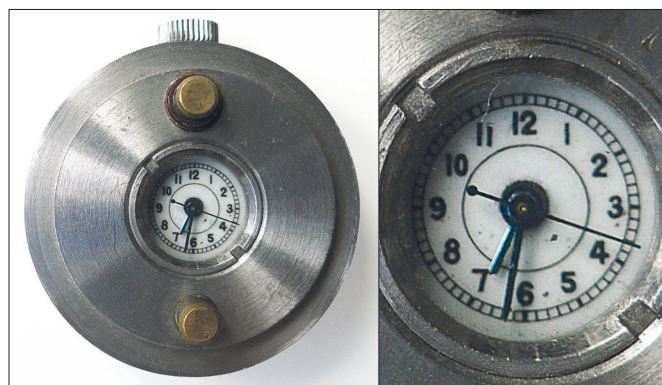
Figure 16A. Dial of an RAF camera watch, 10AF/807.
