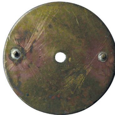
Figure 20. Non-original 'white dial' and 'black dial' made from brass instead of soft iron.
