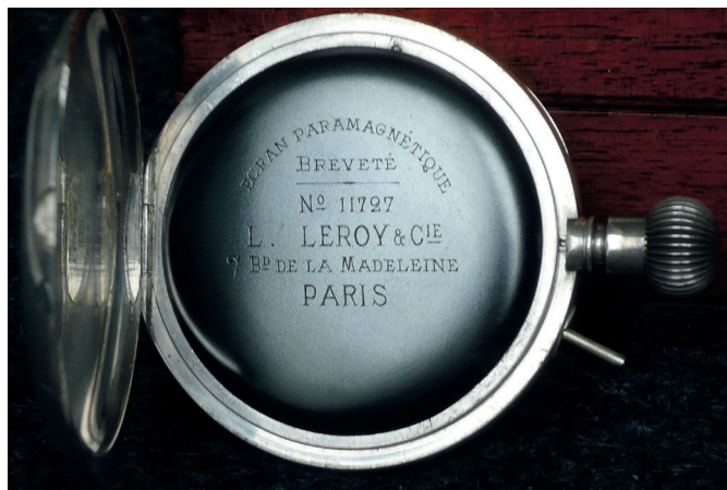
Figure 3A. Soft iron dome of LeRoy Royal Navy Chronometer Watch (CW).
