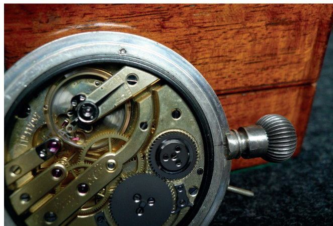
Figure 3B. Soft iron retainer ring of a LeRoy Royal Navy Chronometer Watch (CW) holding the movement. A soft iron plate, not depicted here, is positioned between the dial and the movement.
