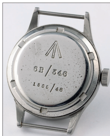
Figure 15. Case back of a Mk. 11, order year 1948, with most of the pittings polished away.
