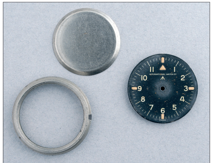
Figure 1. The three parts of the soft iron cage.
