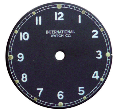
Figure 20. Non-original 'white dial' and 'black dial' made from brass instead of soft iron.
