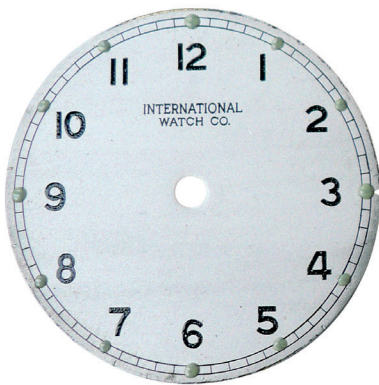
Figure 20. Non-original 'white dial' and 'black dial' made from brass instead of soft iron.
