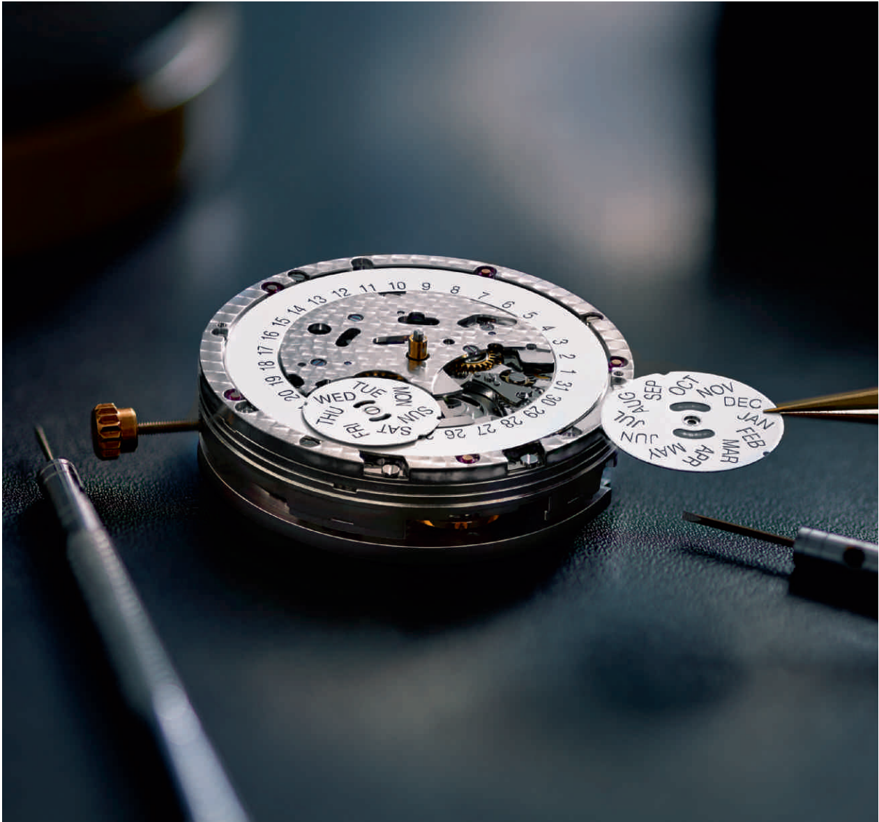
The in-house 52850 calibre shows the month, date and day; the rare combination of an annual calendar and 7-day movement is likely to make this complication from IWC even more interesting for watch connoisseurs
