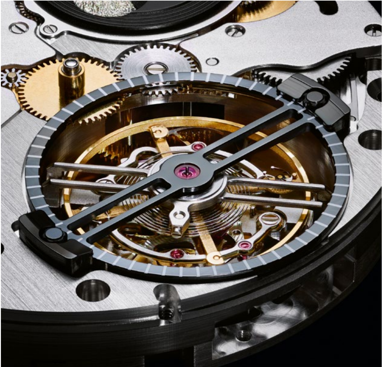
Precision assembly: tourbillon with patented constant-force mechanism
