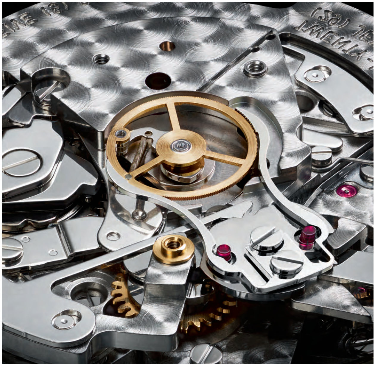
In a rattrapante mechanism, the split-seconds hand starts simultaneously with the stopwatch hand
