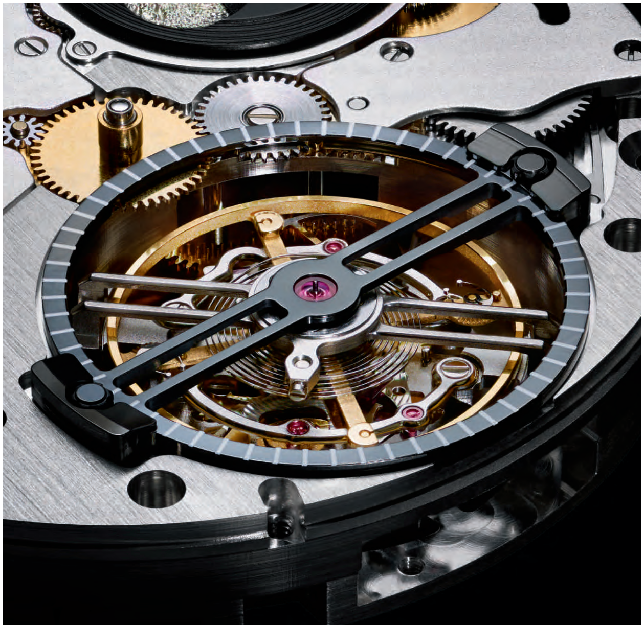
Precision assembly: tourbillon with patented constant-force mechanism
