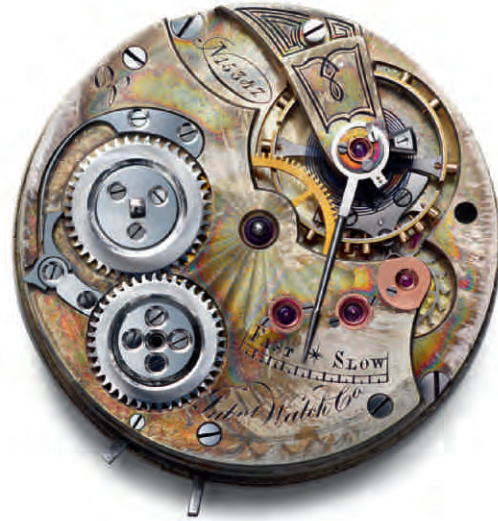
An example of an F. A. Jones calibre, named after IWC's founder, approximately 1875
