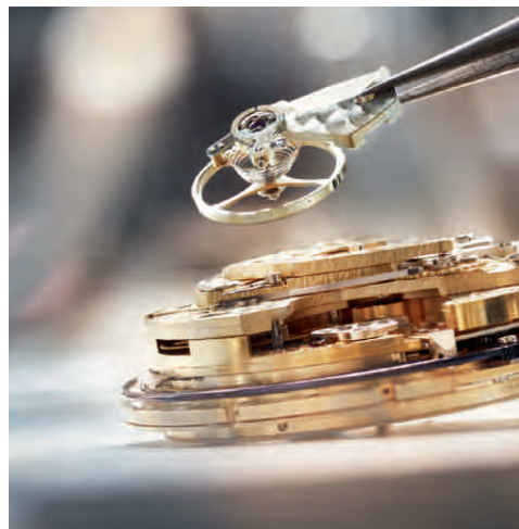
Assembly of the balance spring calls for experience and a steady hand
