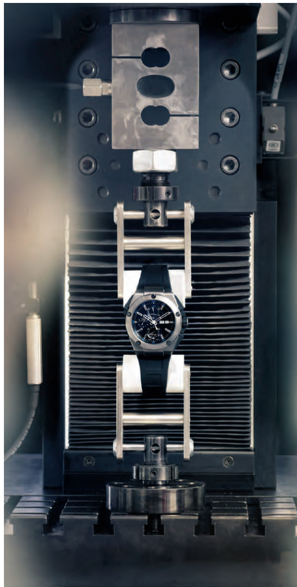
A tensile test ensures that the strap will remain firmly attached to the wearer's wrist even under enormous strains
