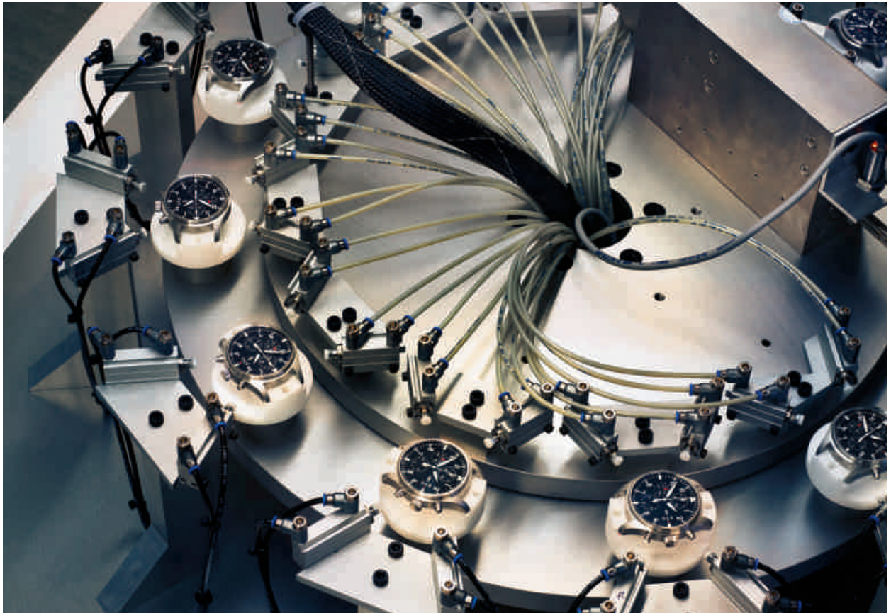
Crown and push-button testing stand: the chronograph mechanism is operated 10,000 times to test its resistance to wear and tear
