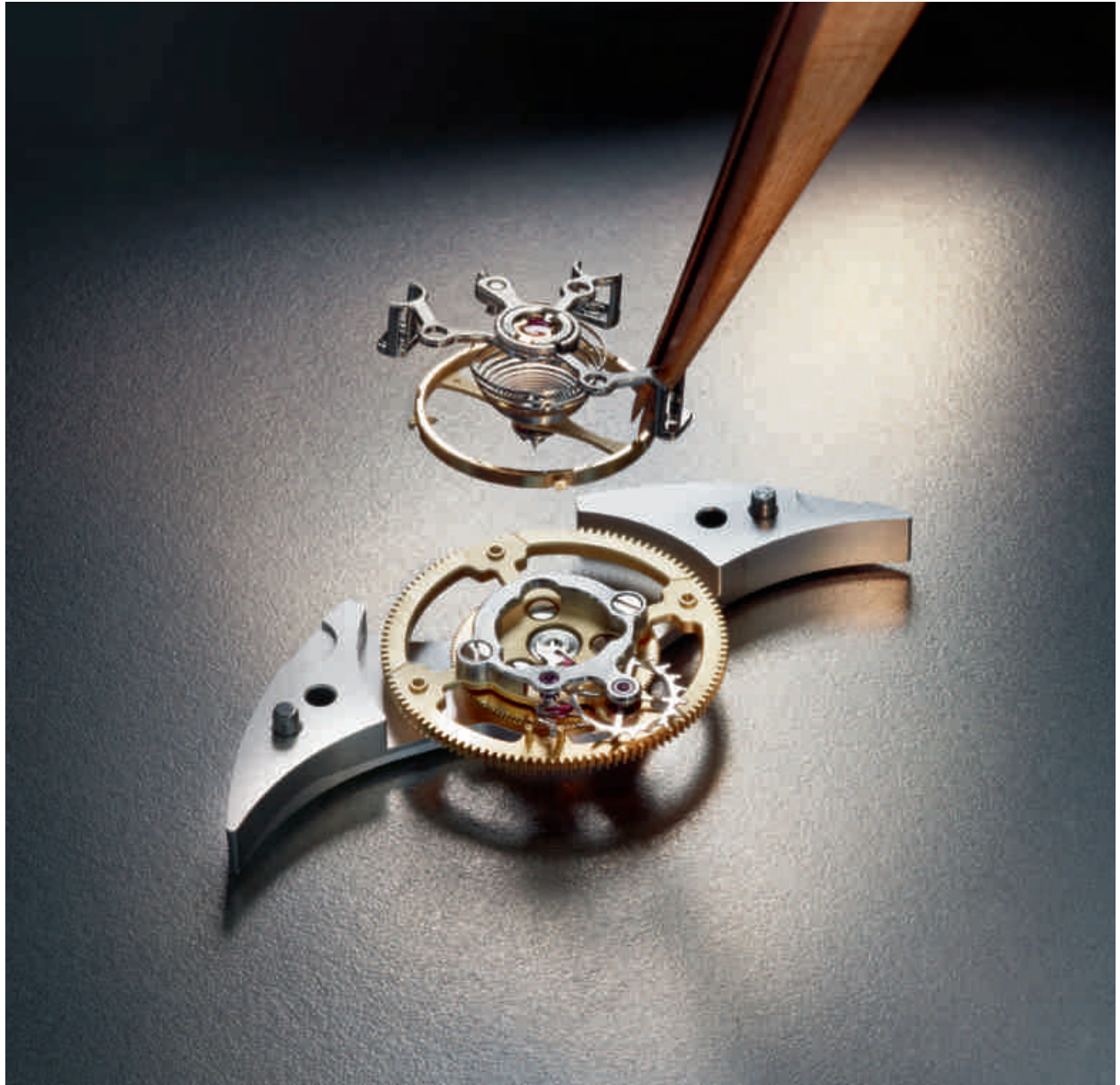
The tourbillon consists of almost 100 tiny parts; assembling them calls for the utmost in concentration
