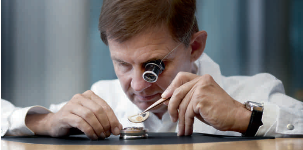
Various skill and precision instruments are the tools an IWC watchmaker uses as he positions the rotor onto the movement
