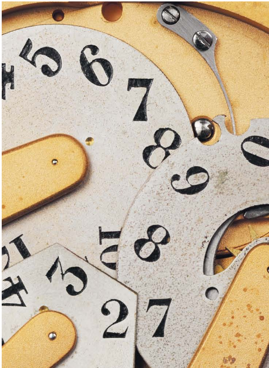
Original hour and minute discs from the Pallweber watch of 1885. With this model, IWC launched the first pocket watch with a perfectly choreographed jumping digital display
