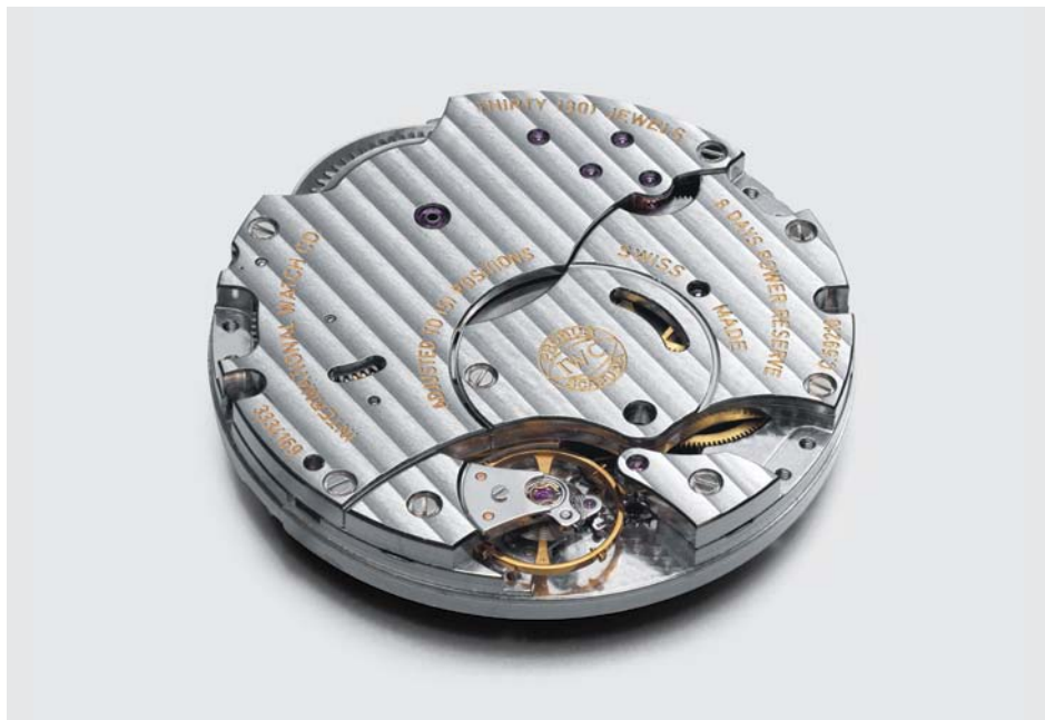
The reverse side of the 59210 calibre. The barrel bridge supports the winding mechanism, barrel and differential, while the display wheel bridge with its “Probus Scafusia” engraving holds the power reserve display
