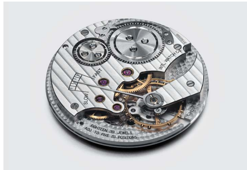
The IWC-manufactured 98295 calibre with design cues from the first F. A. Jones movements: these include an elongated index (the "F. A. Jones arrow"), which facilitates quick, easy adjustment of the spring length, and a three-quarter bridge decorated with Geneva stripes
