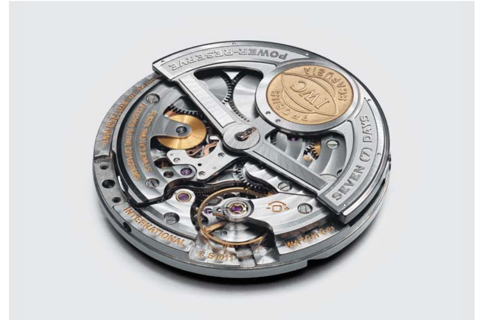
The voluminous, IWC-manufactured 51011 calibre is used in the Portuguese Automatic. With a spring-mounted rotor and Pellaton pawl-winding system it is a member of the 50000-calibre family
