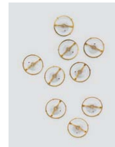
The balance – the beating heart of any mechanical watch
