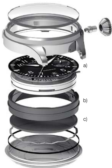
The a) dial, b) casing ring and c) inner back plate of the case form a soft-iron cage
