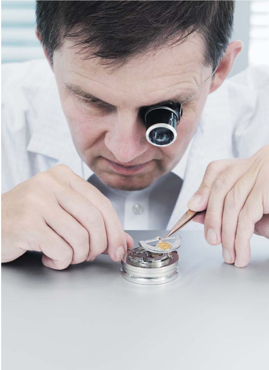
Various skill and precision instruments are the tools an IWC watchmaker uses as he positions the rotor onto the case
