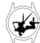
Top: The spring of the date display wheel is tightened via the snail-shaped cam and its rack. After the 31 days have elapsed or – as shown here – by activating the rapid-advance mechanism via the crown, the feeler on the rack jumps from the outer to the inner surface of the cam. The spring is no longer under tension and allows the date hand to jump back to “one”
